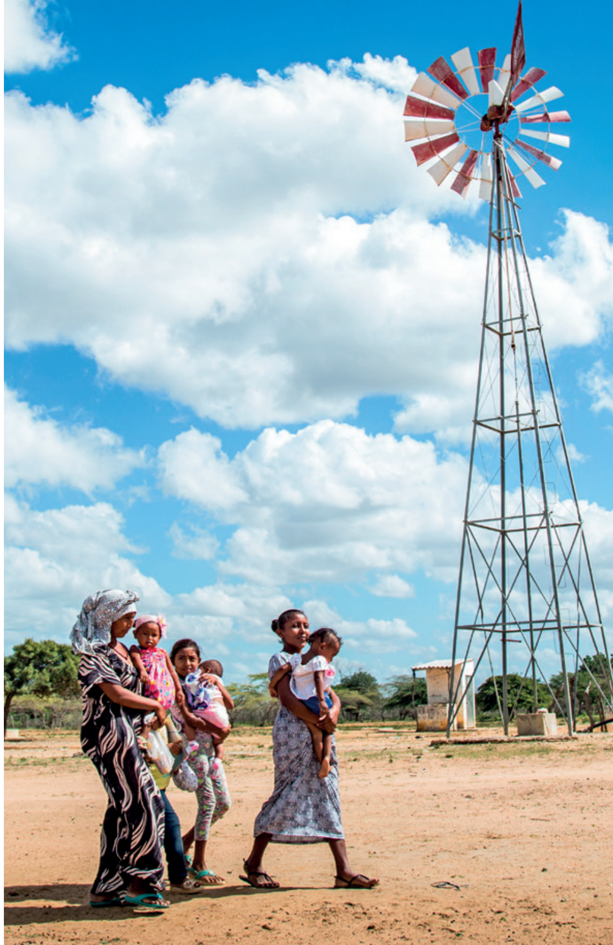
Windmills in the municipality of Manaure (La Guajira) pump water to supply local communities
